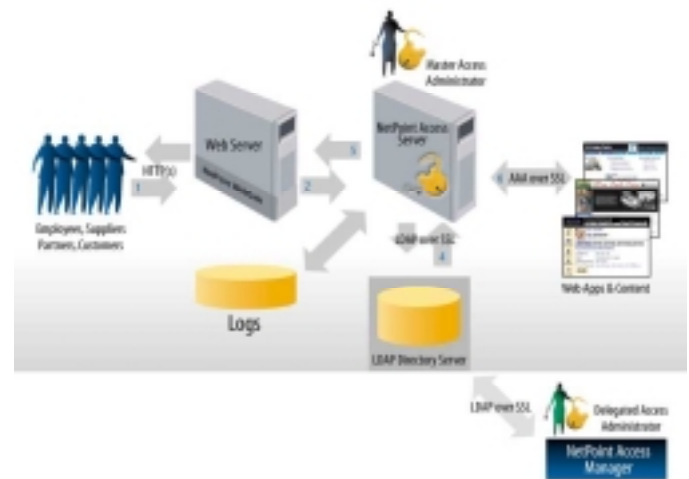
Fig. 3. Sample diagram of a single sign-on solution from Oblix, Inc. [6]
