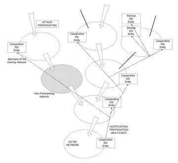
Fig. 1: Example of the infrastructure layout and activation under a DDos attack
