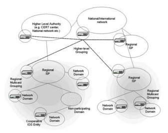
Fig. 3: Multicast grouping of two levels
