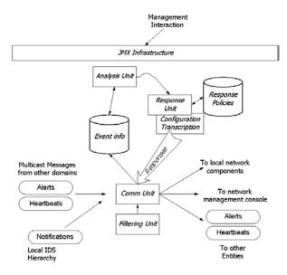
Fig. 2: The software architecture of the IDS Entity
