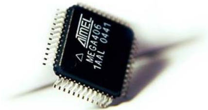
Picture 1.8: ATMEL microprocessor used for digital control of Electrical Drive Systems
