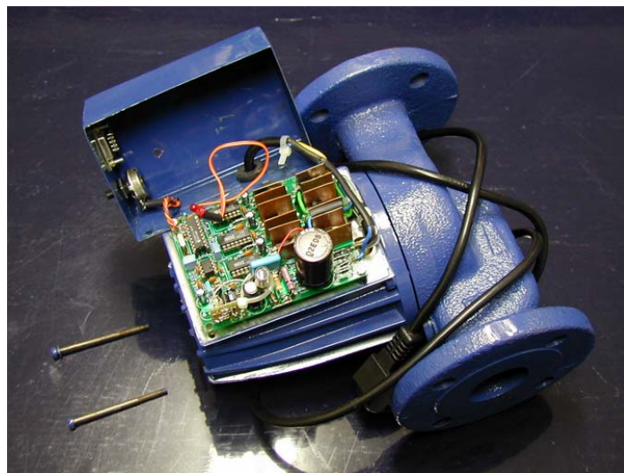
Picture 1.4: Digital Controlled Electric Drive System used as a water pump
