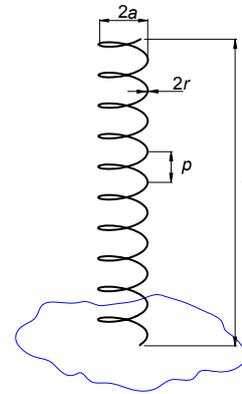
Figure 1. Helical antenna above infinite ground plane.
