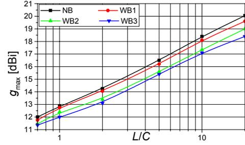
Figure 3. Maximal antenna gain versus normalized antenna length.
